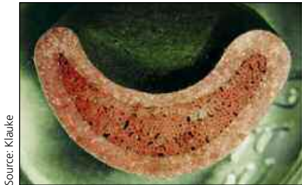
Picture 4: A cross sectional view of an indent crimp (with manufacturers recommended tool) shows the even arrangement of conductor in the lug
