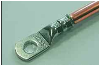
Picture 5: Professional crimp on a solid conductor with matched tube dimension
