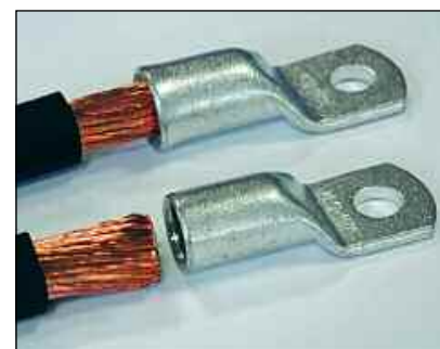
Picture 2: Cable lugs “F type” for fine stranded conductors for easy insertion with no splicing
