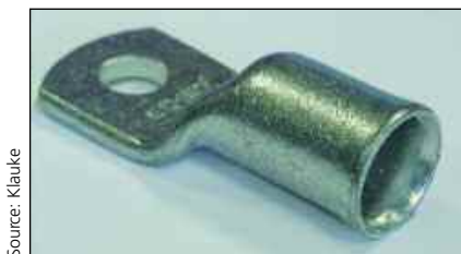
Picture 6: F-Cable lugs with flared entry represent an option when cables of class 5 and 6 will not fit into normal cable lugs.
