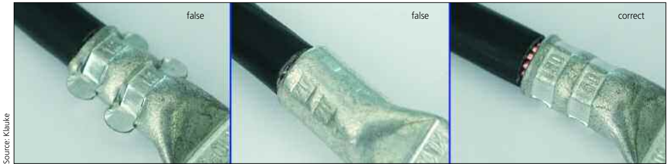
Picture 5: Incorrect and correct crimps in comparison: An incorrect crimp (left: excess crimping, middle: low force crimping, and usage of incorrect crimping tools can result in an increase in joint resistance and may jeopardise the installation; right: correct crimping)
